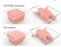
Fig. 13. Artifacts can be seen in the compression due to the lack of deformation DOFs for the bulging effect in MAT-based reduction.
