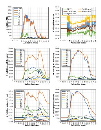
Fig. 16. We plot the detailed benchmarks for BVHs of AABBs and spheres at each individual deformable body in the falling dinosaur animation (Fig. 15). We also compare the culling effectiveness of different bounding primitives in the top-right plot, where **error** is for primitives with the same Hausdorff error, and **num** is for the same numbers of leaf primitives.
