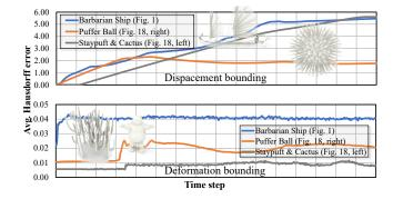
Fig. 19. Average Hausdorff errors of examples in Fig. 1 and Fig. 18. The rest-shape MAT of each model is also given. Due to the large rigid body motion in those examples, displacement bounding yields very high Hausdorff errors (e.g. over 500% of the barbarian ship in Fig. 1). The deformation bounding however produces tight enclosure of deformed model consistently.
