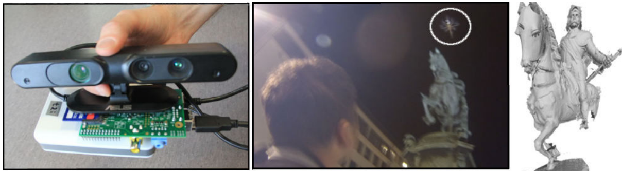
Figure 1: Reconstruction of a statue using a multicopter: (left) handheld ASUS Xtion depth sensor - Raspberry Pi - battery system; (middle) remotely controlled multicopter while recording depth maps; (right) reconstructed 3D model of the statue.
