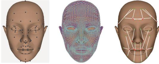
**Fig. 4.** Left. Front view of an input face mesh with MPEG-4 FDPs scattered data set associated. Center. Multi-layered structure representing the skin. Right. The muscle map.
