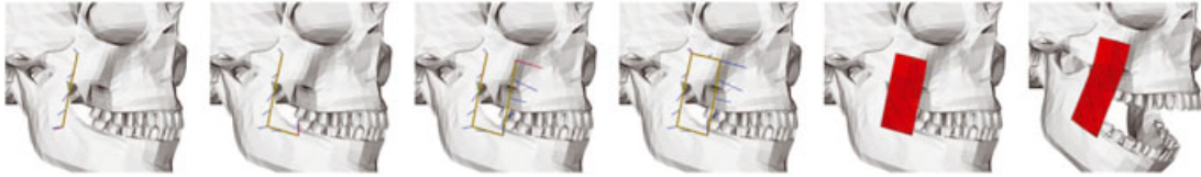
Figure 1. The closed contour C is drawn upon underlying structures, in this case the skull. Then, a hexahedral mesh M is morphed to fit C . M is passively deformed as the skull moves.
